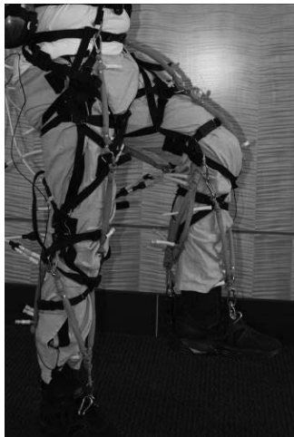
Fig.8. Soft exosuit actuated by pneumatic actuator.
