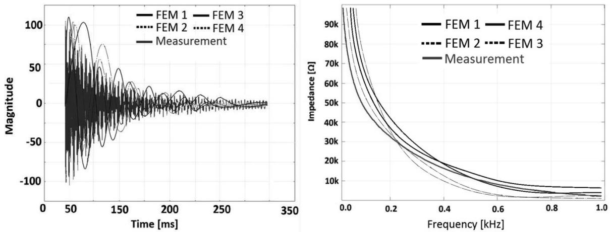
**Fig. 3** Comparison of experimental input signal and FEM model for composite sample: Dependence of FEM model convergence on degree of adaptive network (left), Comparison of measurement and FEM model of impedance dependence on the frequency of alumina plate (right).
