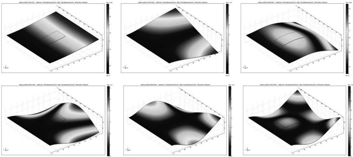
**Fig.5** FEM distribution of total deformation for each mode of vibrations (1-6 mode of vibrations).
