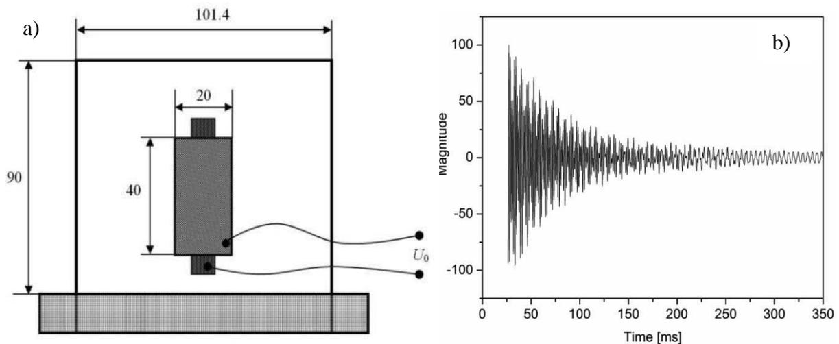
**Fig. 1** Dimensions of vibrating plate from carbon composite with thin piezoelectric rectangular plate (left), An mechanical pulse excitation (right).
