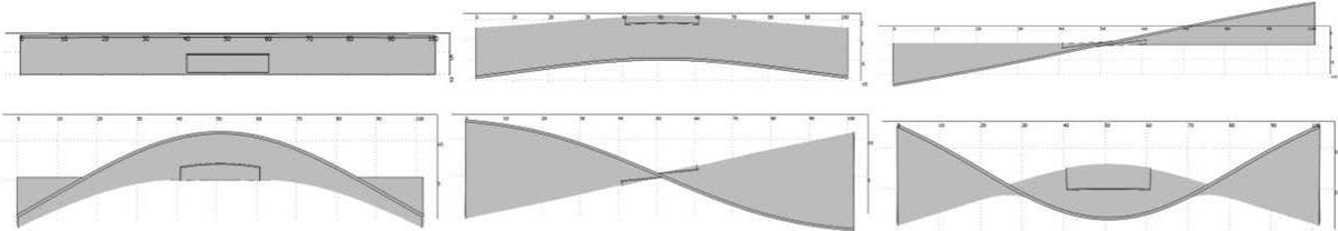
**Fig.4** FEM shape mode of composite plate with piezoceramics sensor (1-6 mode).
