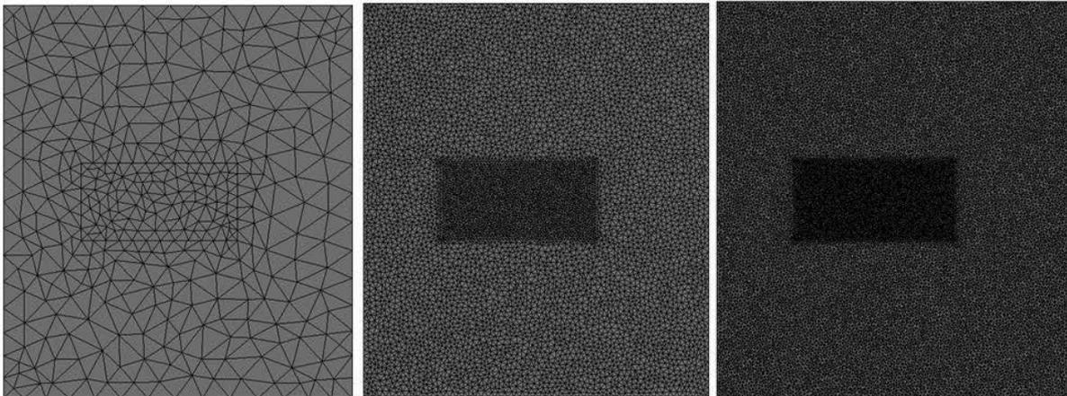
**Fig. 2** FE meshing of the model in the calculation convergence: Adaptive meshing for the minimization of the residues in the solved area.
