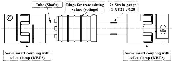
Fig. 4 3D model of measuring sensor with couplings.
