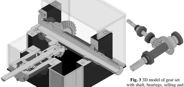
Fig. 2 3D model of gearbox for testing of bevel gears.
