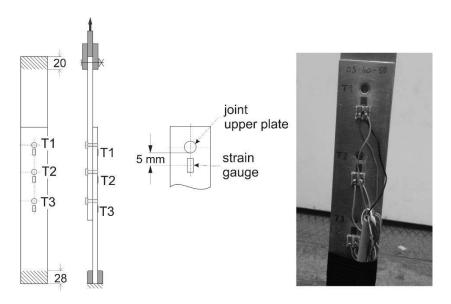
Fig. 2 Scheme and real sample of tested specimen
