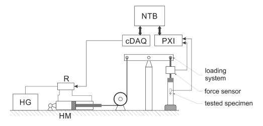
Fig. 3 Scheme of the testing stand
