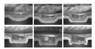
**Fig. 1** Creation of the round clinched joint (www.tox-de.com)
