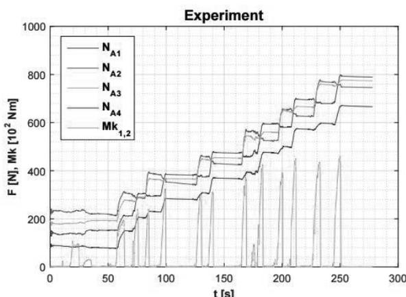
**Fig. 4** The data (Forces and Tightening torque) measured over time.
