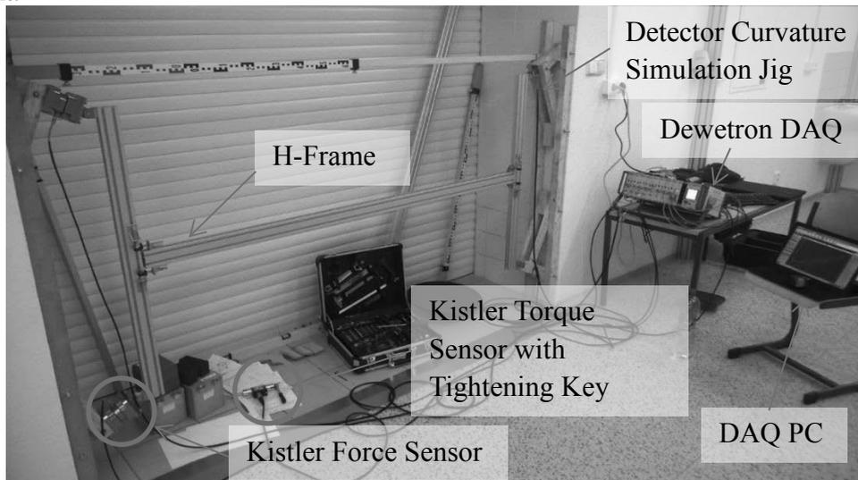
**Fig. 3** Experimental measurement of the welding support in the Laboratory of Extreme Loading.
