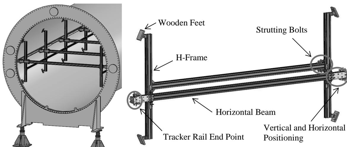
**Fig. 1** Installation of the tool in the housing of the inner detector.
