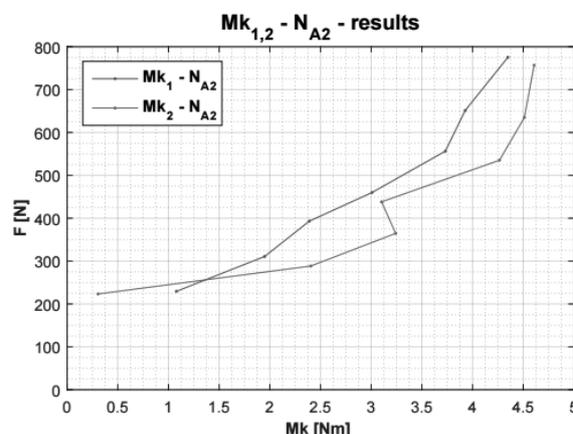
**Fig. 5** The contact forces in dependence on tightening torque.
