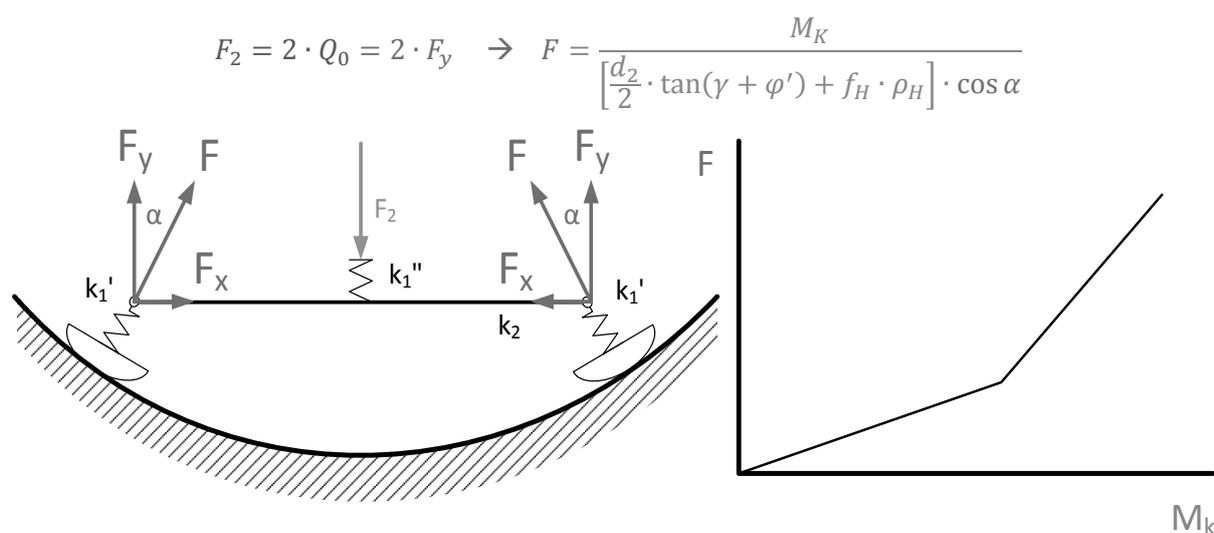
**Fig. 6** Mathematical model of the structure stiffness changes
