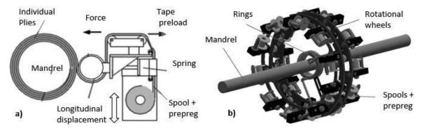
Fig. 1 The used manufacturing methods a) Wrapping b) Winding
