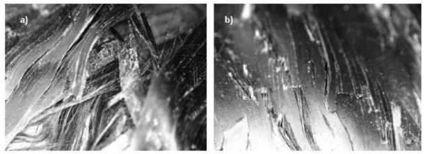
Fig. 5 The found typical failures of parts in bending test explored for the a) wrapped b) winded, parts
