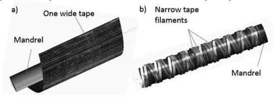
Fig. 2 The two principles how the fiber material is layered a) Wrapped b) Winded
