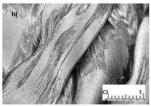
Fig. 3 The surface of the a) wrapped b) winded, parts from carbon prepreg (added scale 1 cm)
