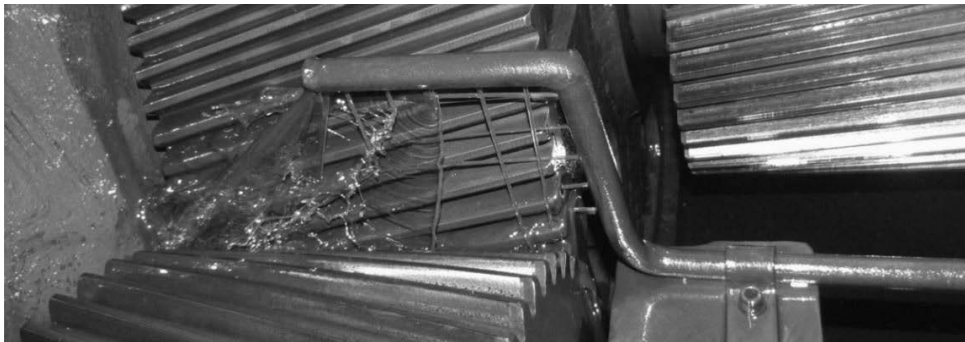
Fig. 6 Splash lubrication with the opposite direction of rotation
