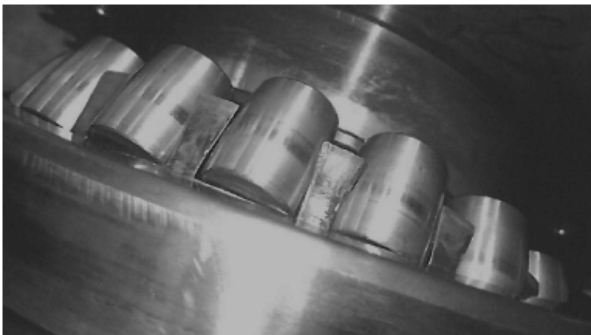
Fig. 6 Damaged input shaft bearing on the engine side
