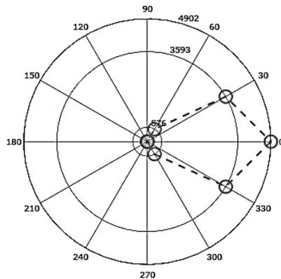
**Fig. 2** Roller load distribution
