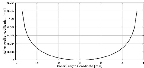
**Fig. 5** Roller profile modification
