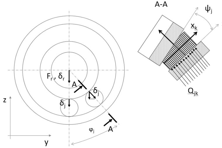
**Fig. 1** Coordinates of bearing model (ISO, 2008)
