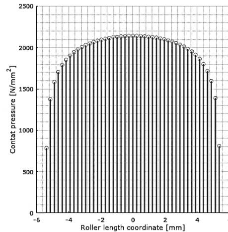
**Fig. 3** Roller contact pressure distribution
