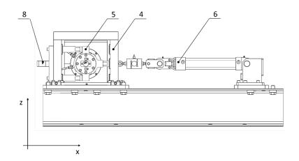
Fig. 2 Test rig front view with highlighted tested bearing housing
