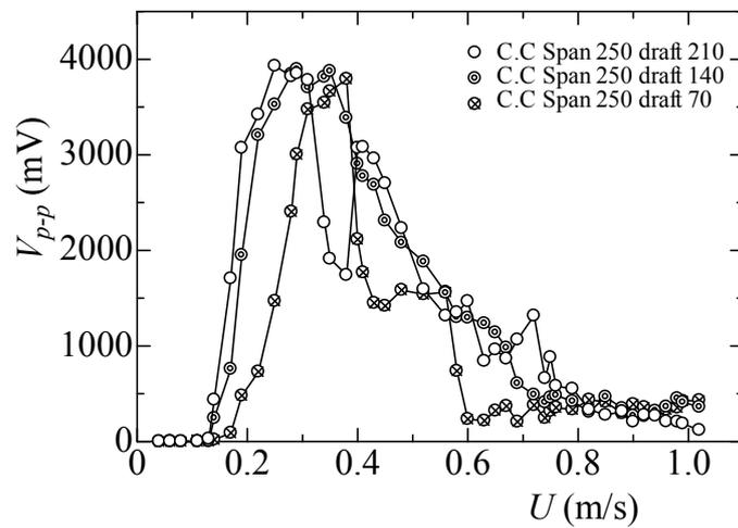
**Fig. 8** Relationship between flow velocity and output voltage, in the case of sharp square cylinder
