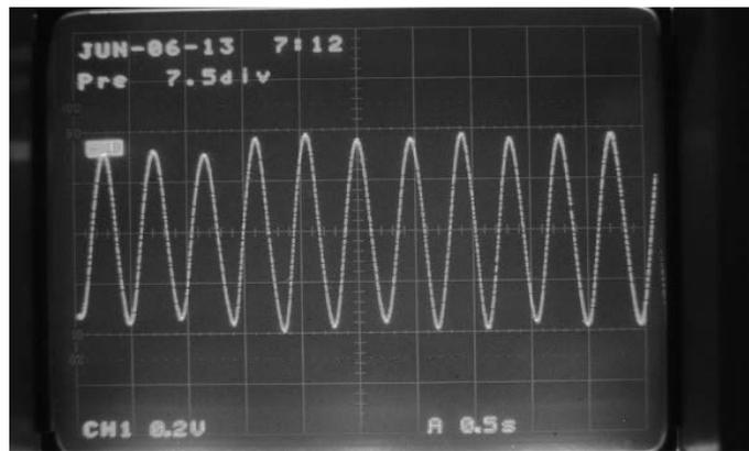
**Fig. 5** An example of the output waveform from the power generation object
