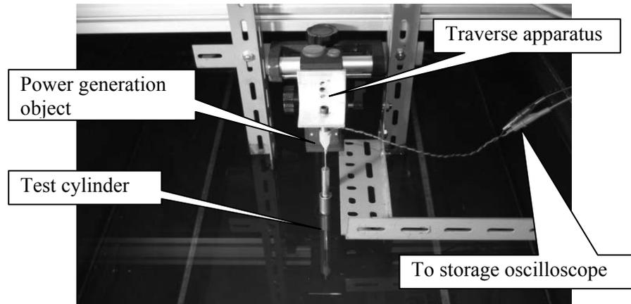
**Fig. 4** The photograph of the situation where the test cylinder was set in the traverse apparatus
