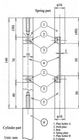
**Fig. 1** The schematic drawing of a test cylinder spring section
