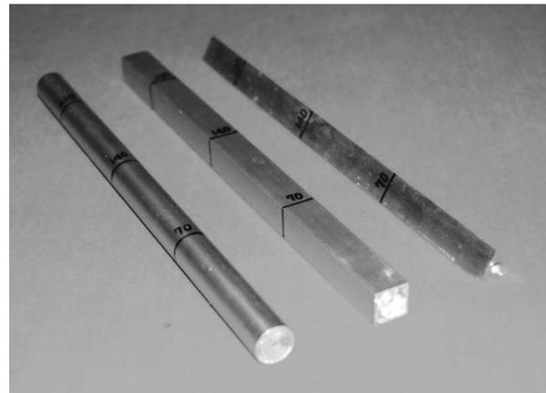
**Fig. 2** Body section shape of the test cylinder (circular cylinder, square cylinder, and triangular cylinder)
