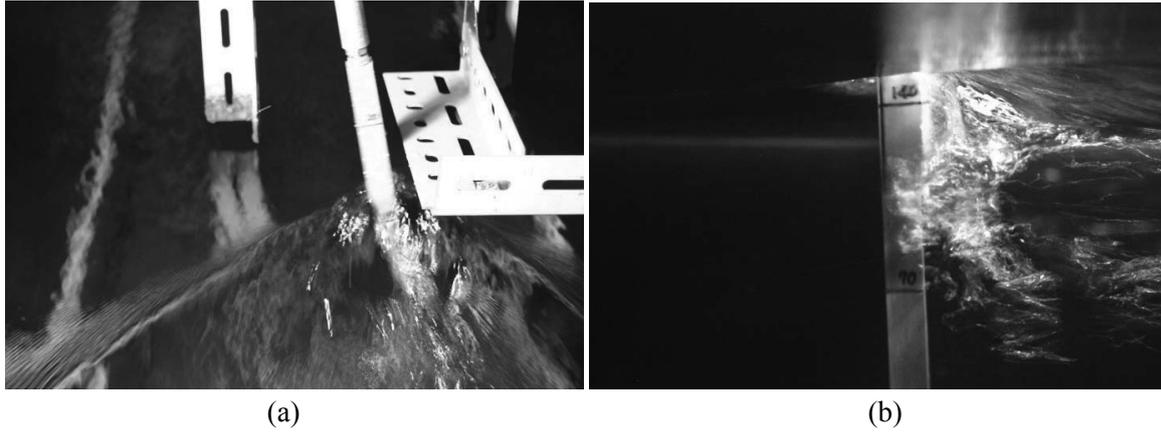
**Fig. 7** The behavior of the plane square cylinder, and the aspect of flow; the span of the square cylinder was 250 mm, and the submersion depth was 150 mm, (a) the photograph seen from the down stream side, (b) the underwater photograph seen from the width side
