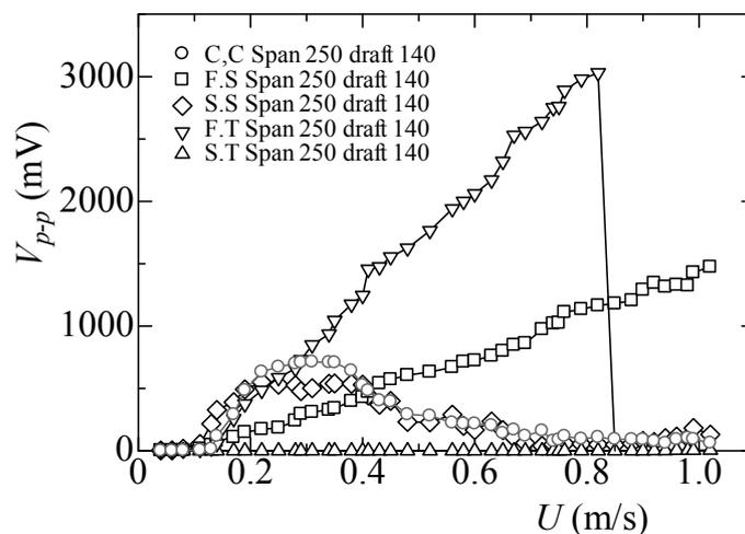
**Fig. 6** Relationship between flow velocity and output voltage, in the case of circular cylinder
