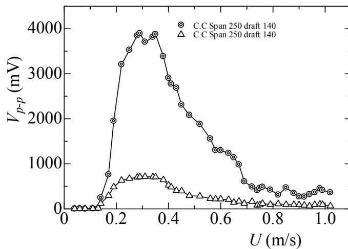
**Fig. 9** Relationship between flow velocity and output voltage, in the case of flat square cylinder
