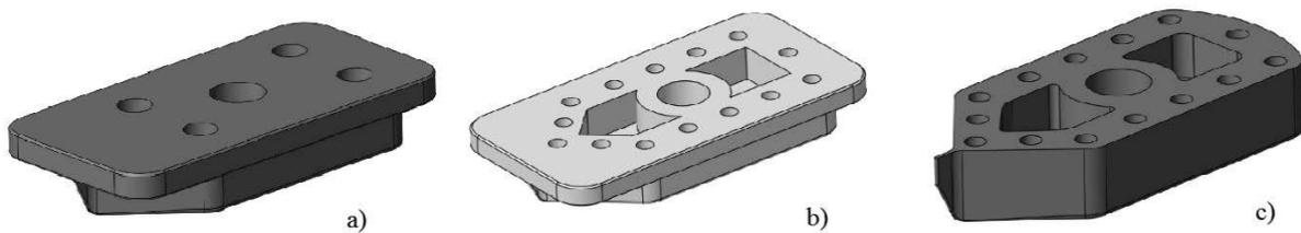
**Fig. 4** Changes of shape and mass of punch
