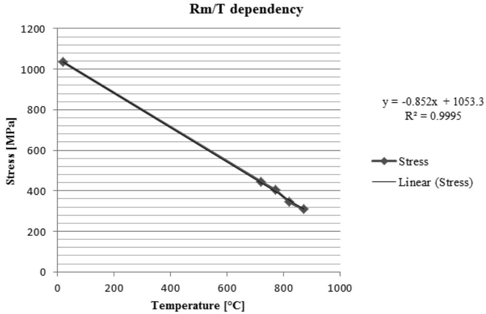
Fig. 1 Graph of Rm/T dependency of molybdenum
