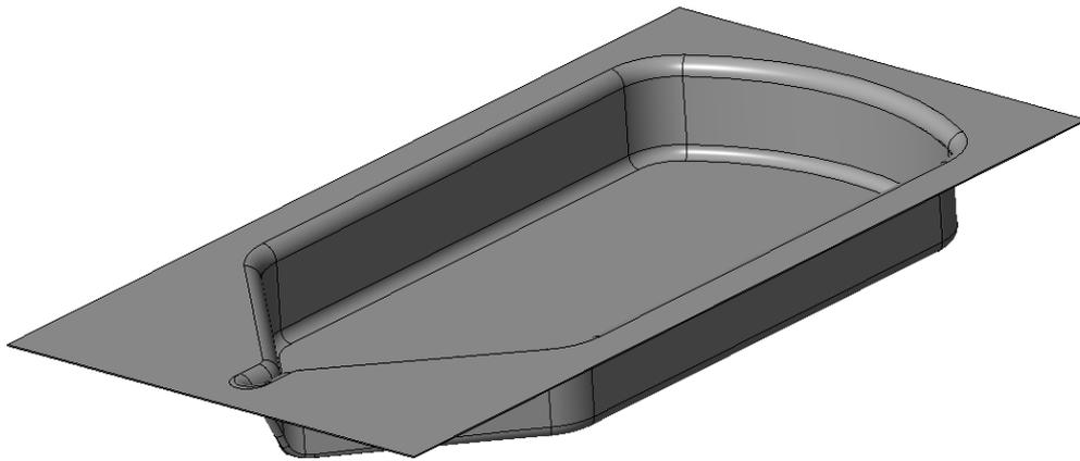
**Fig. 3** 3D CAD model of molybdenum sheet shaped into the finally form
