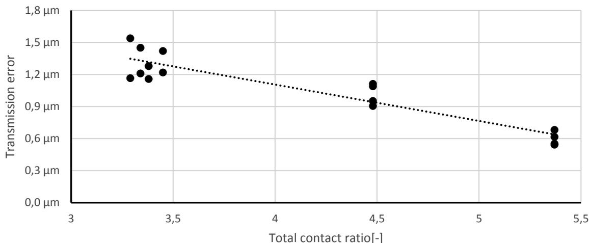
**Fig. 6** Graph of Transmission error to total contact ratio
