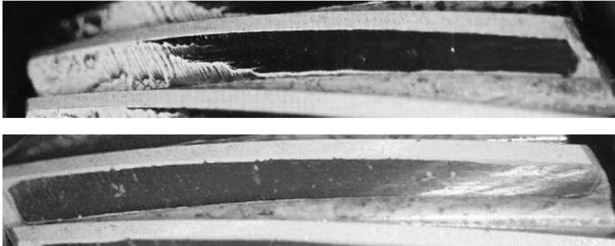
**Fig. 2** Footprint of the gear pair 1
