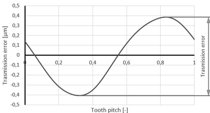
**Fig. 4** Peak to peak transmission error
