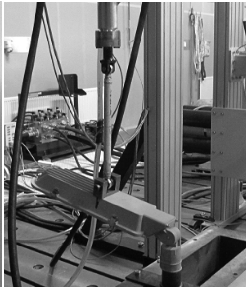
Fig.3 Loading of the luminaire
