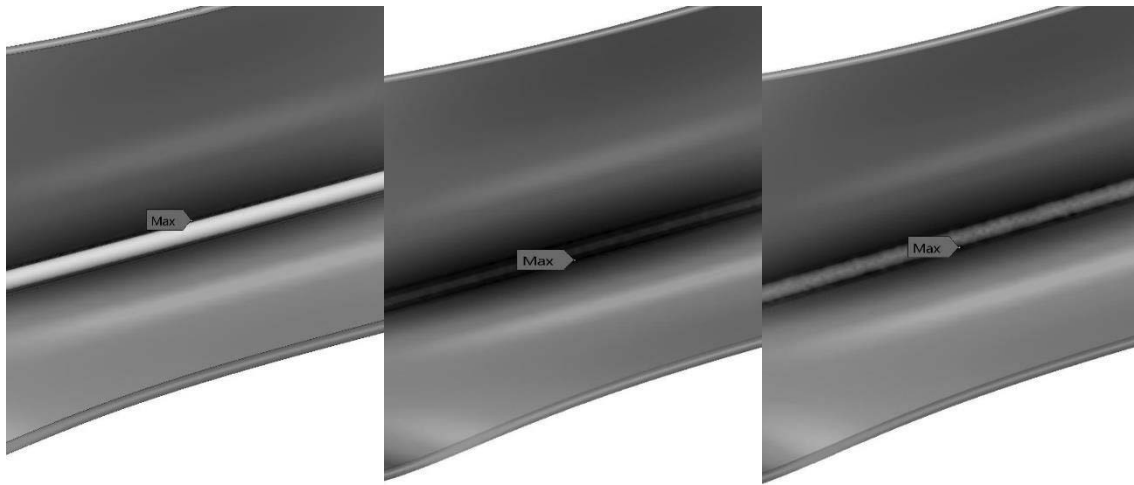
Fig. 3 Different corner welds, left - convex, middle - flat, right – concave
