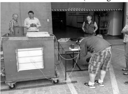
Fig. 4 c Processing the flap door test and flame ignition
