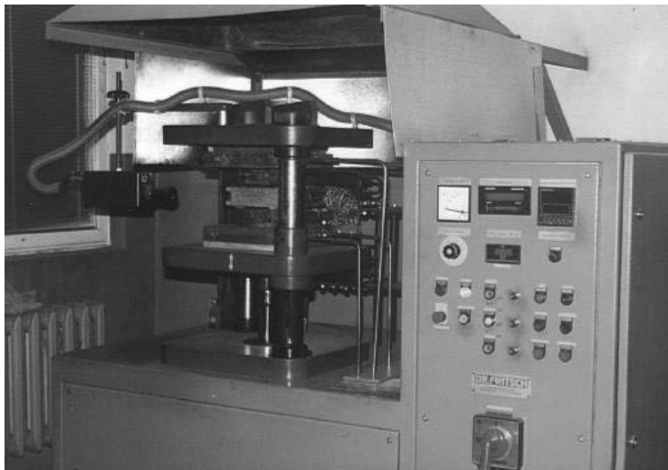
Fig. 1 Hot pressing operation carried out in air
