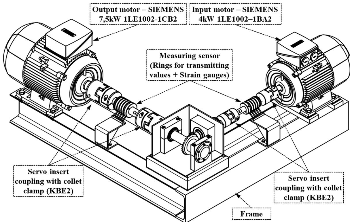
**Fig. 5** 3D model of test rig for testing of bevel gears.
