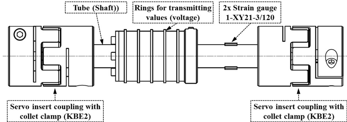
**Fig. 4** 3D model of measuring sensor with couplings.
