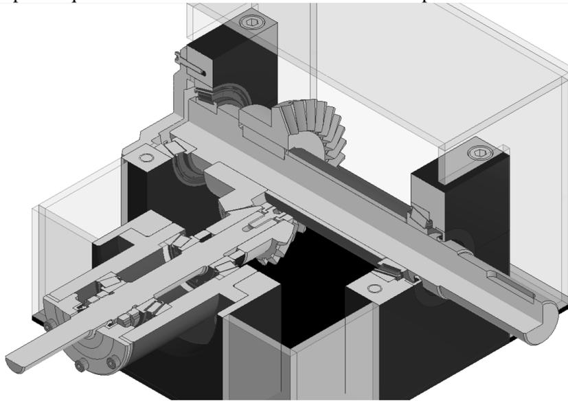
**Fig. 2** 3D model of gearbox for testing of bevel gears.
