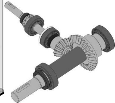
**Fig. 3** 3D model of gear set with shaft, bearings, selling and axial locking.
