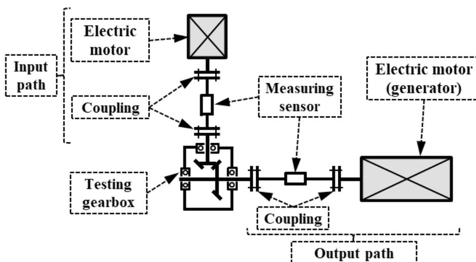
**Fig. 1** Conceptual scheme of electrically close loop for testing of bevel gear.
