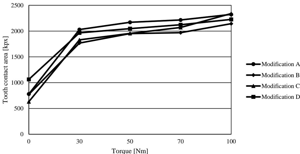
**Fig. 2** Measured data of increasing tooth contact area depending on torque
