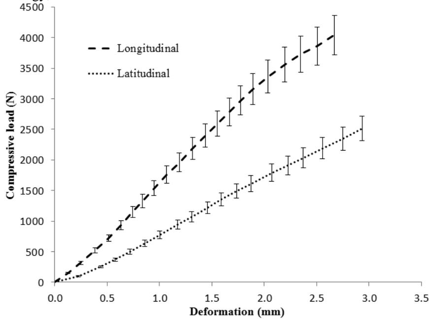
**Fig. 3** Relationship between compression force and deformation of coconuts in two directions
