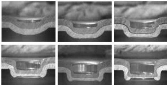
**Fig. 1** Creation of the round clinched joint ([www.tox-de.com](http://www.tox-de.com))
