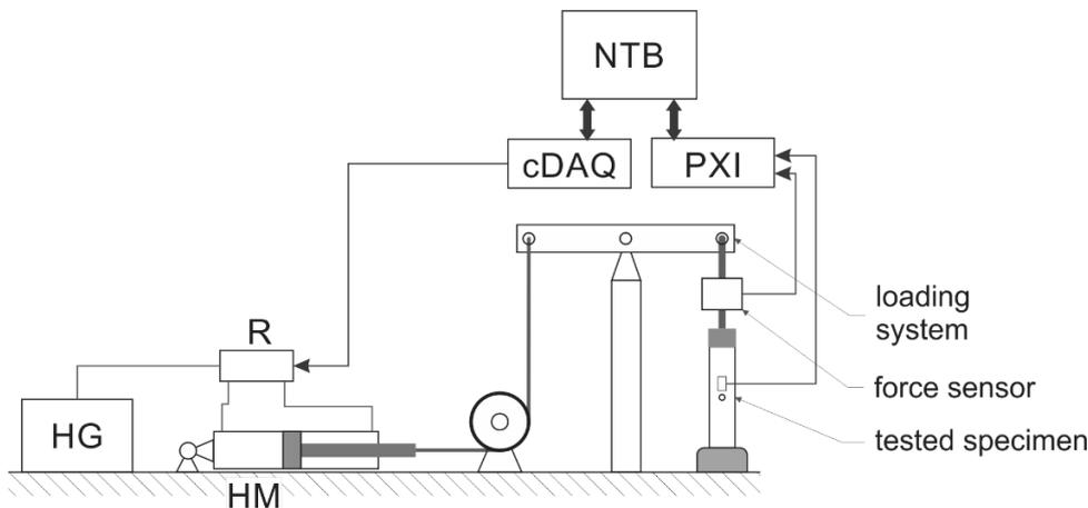
**Fig. 3** Scheme of the testing stand
