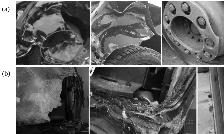
Fig. 5 Characteristic damage in a form of truck hub cap shape mapping on the passenger car fender and paint layers from that hub cap (a) and bark identified in the road tractor cabin (b).
