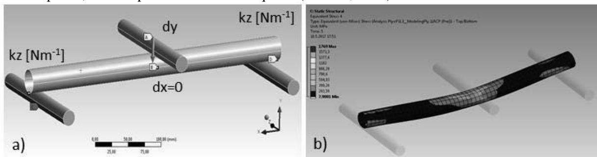
**Fig. 4** The numerical model of shell composite bending test a) scheme with the boundary conditions b) An example of resulting stress in one ply
