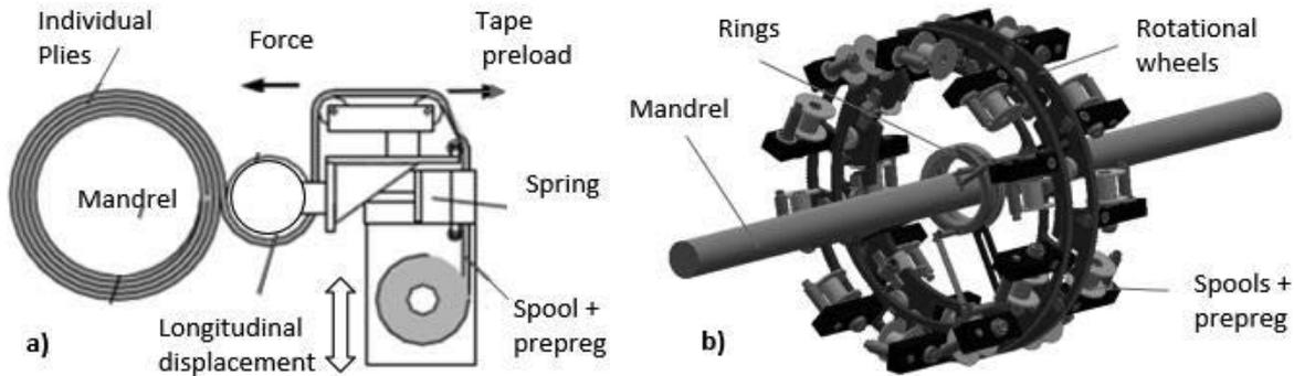
**Fig. 1** The used manufacturing methods a) Wrapping b) Winding
