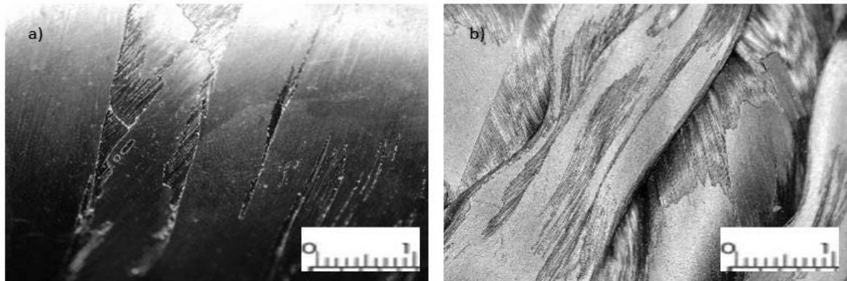
**Fig. 3** The surface of the a) wrapped b) wound, parts from carbon prepreg (added scale 1 cm)
