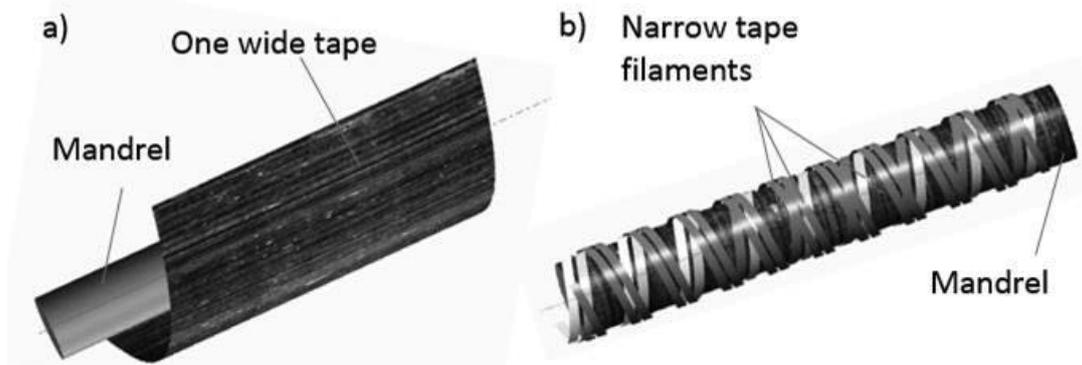
**Fig. 2** The two principles how the fiber material is layered a) Wrapped b) Winded
