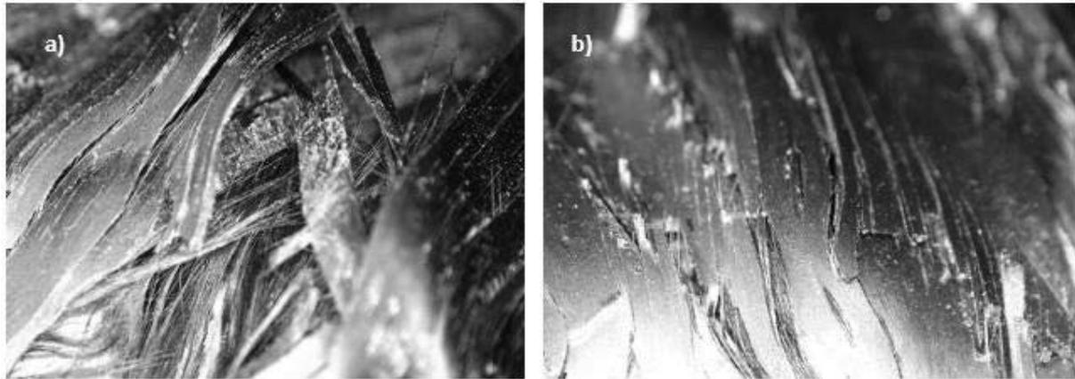
**Fig. 5** The found typical failures of parts in bending test explored for the a) wrapped b) winded, parts
