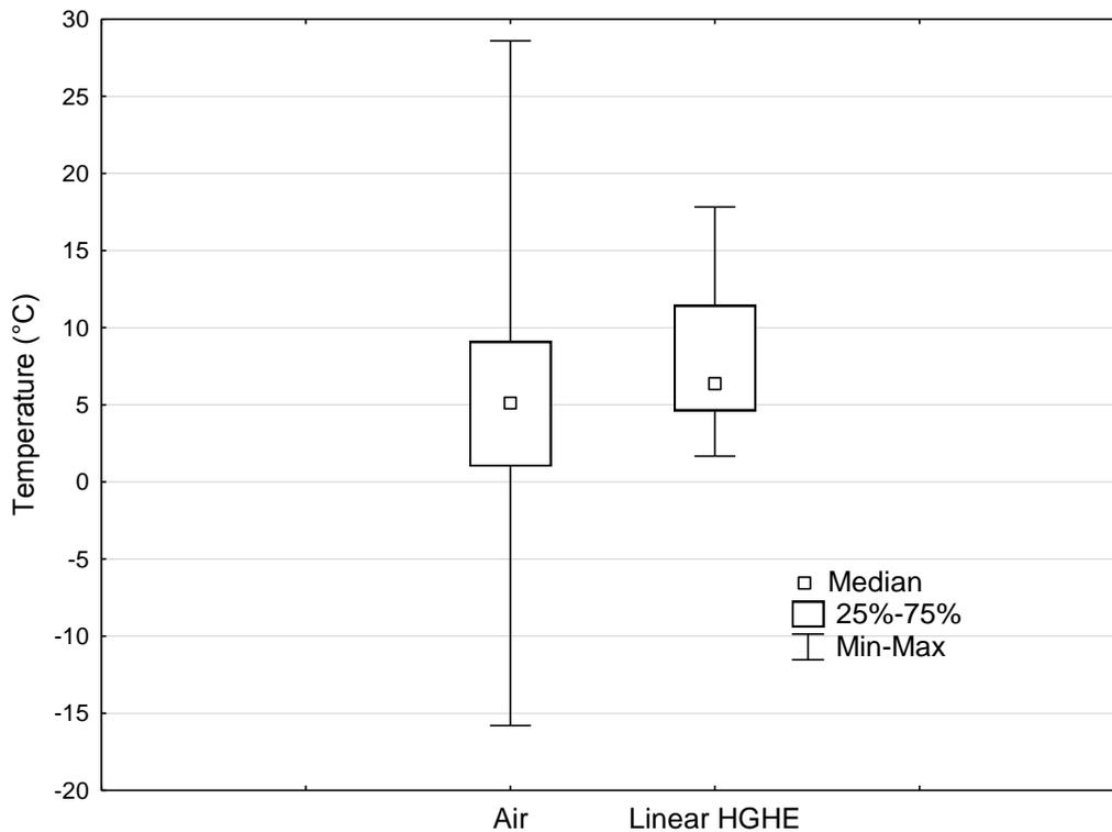
**Fig. 1** Box-whisker plots of temperatures of the low-temperature sources
