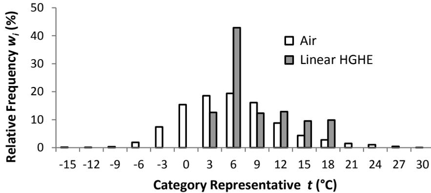
**Fig. 2** Histograms of temperature relative frequencies in low-temperature sources
