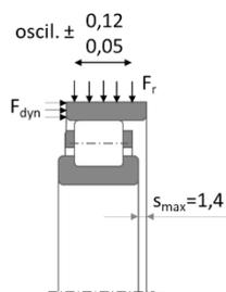
Fig 1. Studied roller bearing with free axial play of outer ring and its predicted axial oscillation during dynamic loading.
