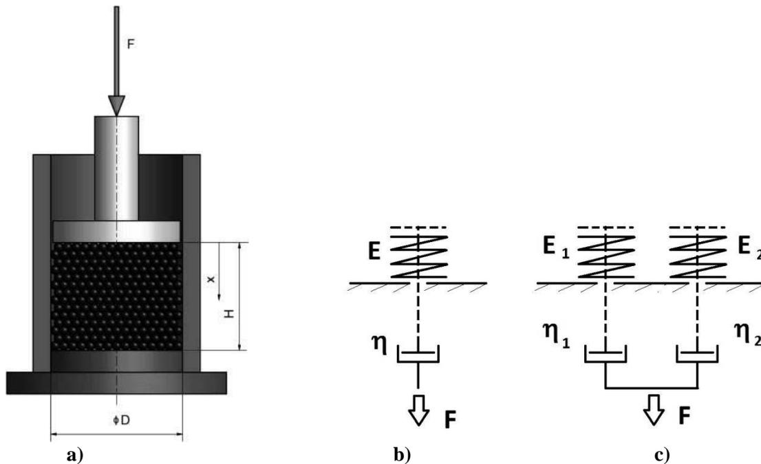
**Fig. 1** a) Scheme of pressing equipment; b) Scheme of one branch model; c) Scheme of two branches model
