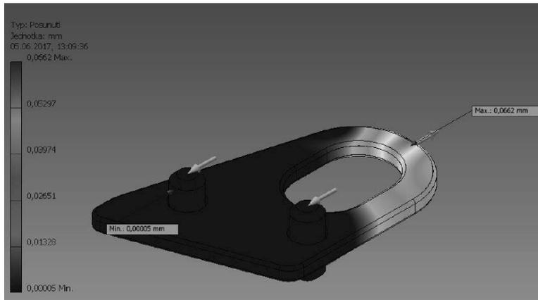
**Fig. 5** The calculation of the overall displacement in program Autodesk Inventor Profesional
