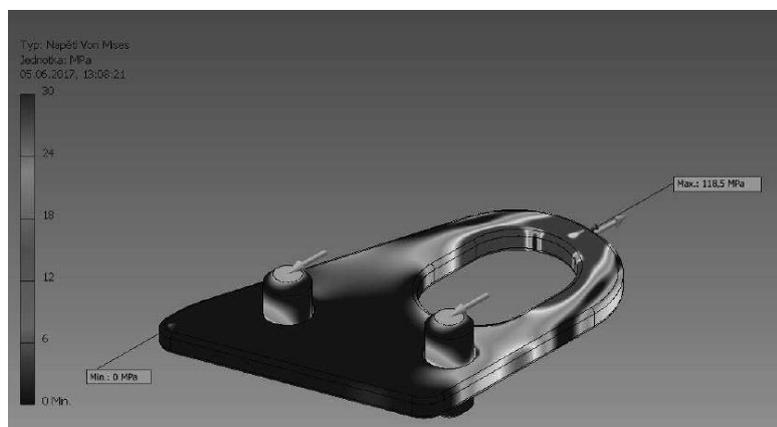
**Fig. 4** The calculation of over tensions in the program Autodesk Inventor Profesional (Tension von Mises)
