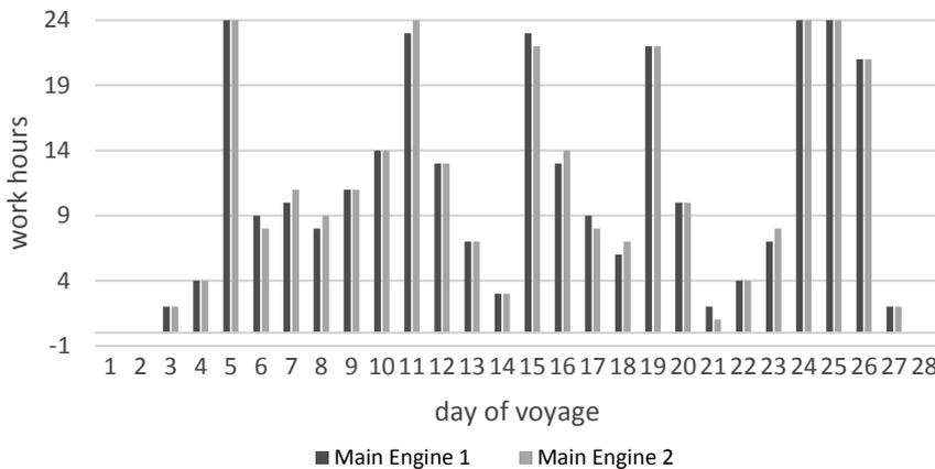
**Fig. 3** Work hours of main engines during operational tasks
