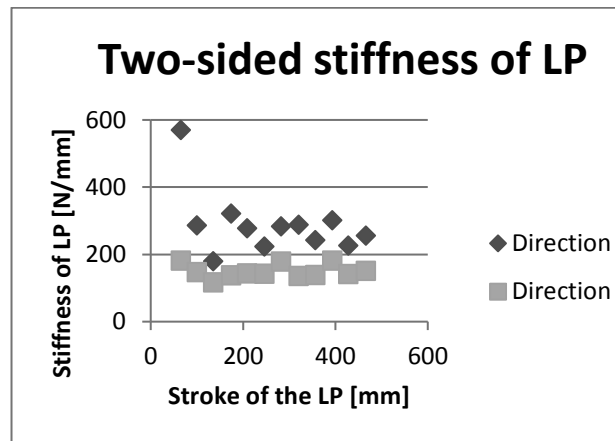
Fig. 6 Two-sided stiffness of linear positioner ( Klíma,2016 )
