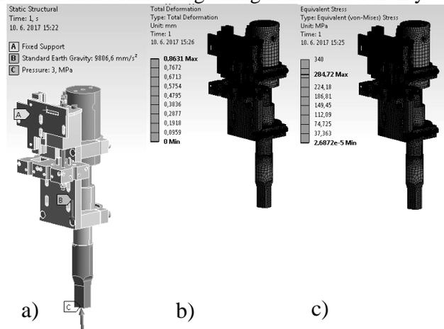
**Fig. 4** a) Gripping and loadings, Variant no. 3; b) Deflection of the sonotrode head, Variant no.3; c) Maximum strength in Variant no. 3;
