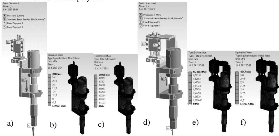
**Fig. 2** a) Gripping and loadings, Variant no.1; b) Deflection of the sonotrode head, Variant no.1; c) Maximum stress in Variant no.1; d) Gripping and loadings, Variant no.2; e) Deflection of the sonotrode head, Variant no.2; f) Maximum stress in Variant no.2;
