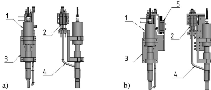
**Fig. 1** a) Welding head gripping, Variant no.1; b) Welding head gripping, Variant no.2; (1) Sonotrode, (2) Linear conduct, (3) Pneumatic cylinder, (4) Cooling tube, (5) Gripping construction
